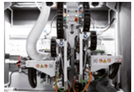
High-power trimming unit SF30 with automatic adjustments
