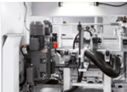
Optional extension for the application of edge sealing or chamfer lacquering
