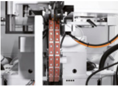
Tension-free infeed system with improved stability
