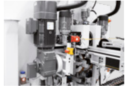
Frequency or servo-controlled drive systems ensure a steady feed rate at all speeds with TENONTEQ D-600 (optional transverse processing)
