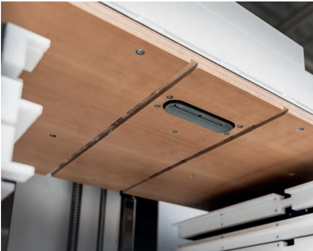
Vacuum suction in the vertical pressure beam
