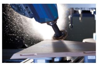
On the new CENTATEQ P-210, the user can select between three-, fourand five-axis heads, and now a gluing function is also possible.
