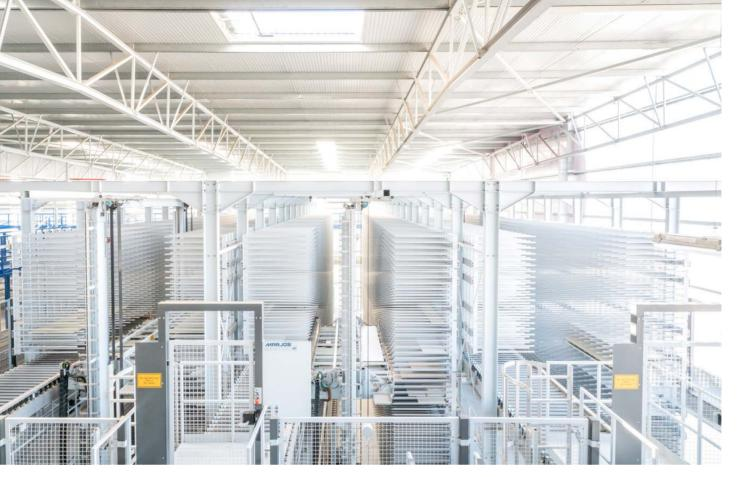
Infinite extension: the gigantic sorting buffer is also a transport lift in the lower level of the production line.
